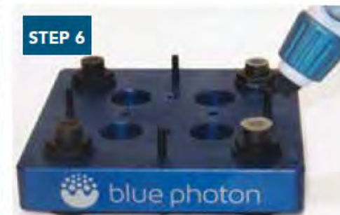
Remove and peel away residual adhesive with steam or hot water spray.
