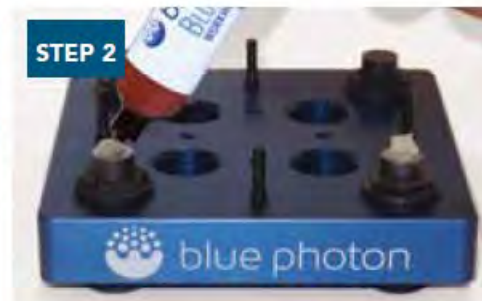
Apply enough adhesive to the grippers to fully fill the gap between the part and gripper.
