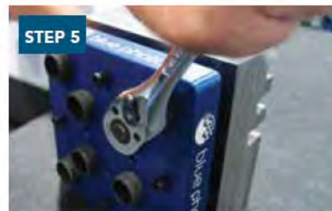
Separate fixture from workpiece with a 1/4 turn twist or hot water soak.
