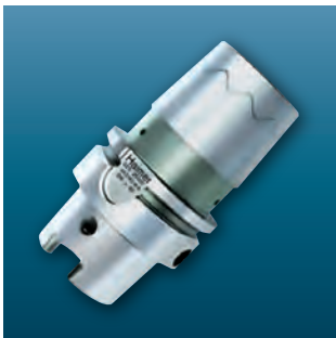
DIN 69893-1 HSK-A63/100, 重型燒結刀桿, HEAVY DUTY CHUCK 夾持直徑16~50mm, 有效長85~200mm, 側邊出水孔
