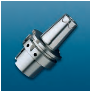
DIN 69893-1 HSK-A63/100, 強力燒結刀桿, POWER SHRINK FIT CHUCK 夾持直徑6~32mm, 有效長70~200mm, 側邊出水孔
